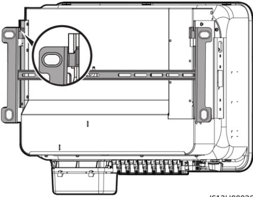
3. Tighten the security Torx screws on both sides.
