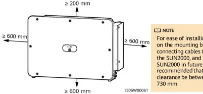
For ease of installing the SUN2000 on the mounting bracket, connecting cables to the bottom of the SUN2000, and maintaining the SUN2000 in future, it is recommended that the bottom clearance be between 600 mm and
