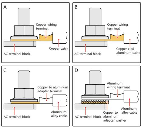
Figure 5-4 Requirements for the OT/DT terminal
