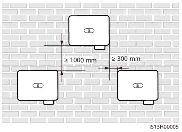
Figure 4-5 Three-layer triangle installation (not recommended)
