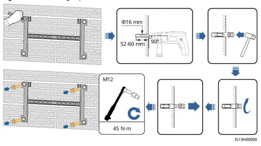
Figure 4-15 Installing expansion bolts
