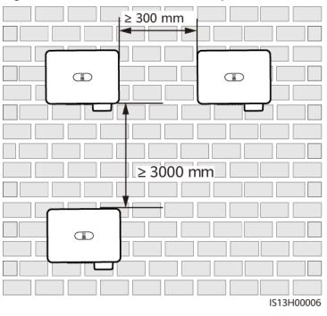
Figure 4-6 Wall-mounted dual-track spaced installation (not recommended)
