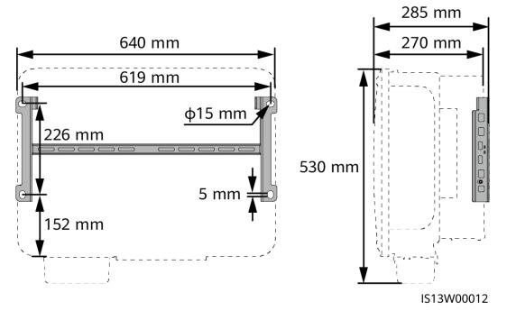
Figure 4-12 Mounting bracket dimensions
