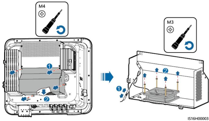
**Step 2** Install a new fan, connect and bind the cables, and install the fan cover.
