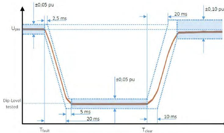
Fig. 4-26: Tolerances for voltage drop tests [2]
