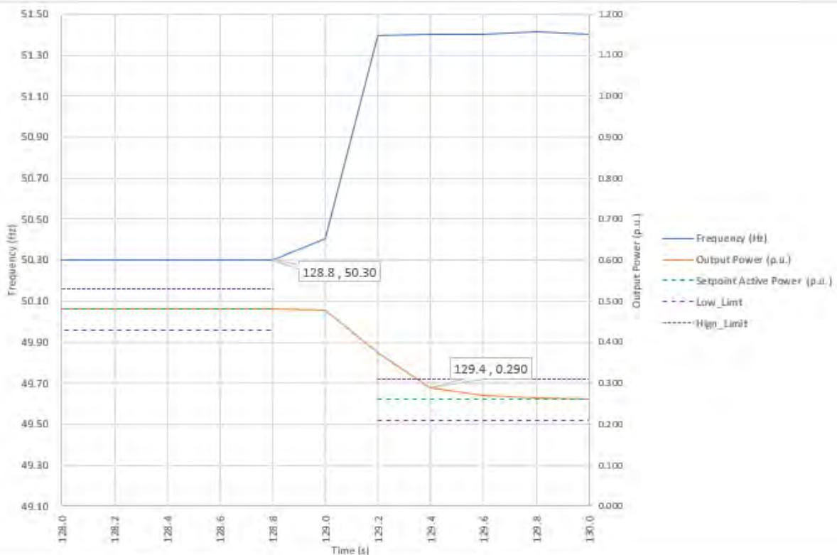
dP(f) desired: 40.0% P<sub>ref</sub>/HzdP(f) measured: 40.0% P<sub>ref</sub>/Hz**Power gradient (Step 3 to 4)**
