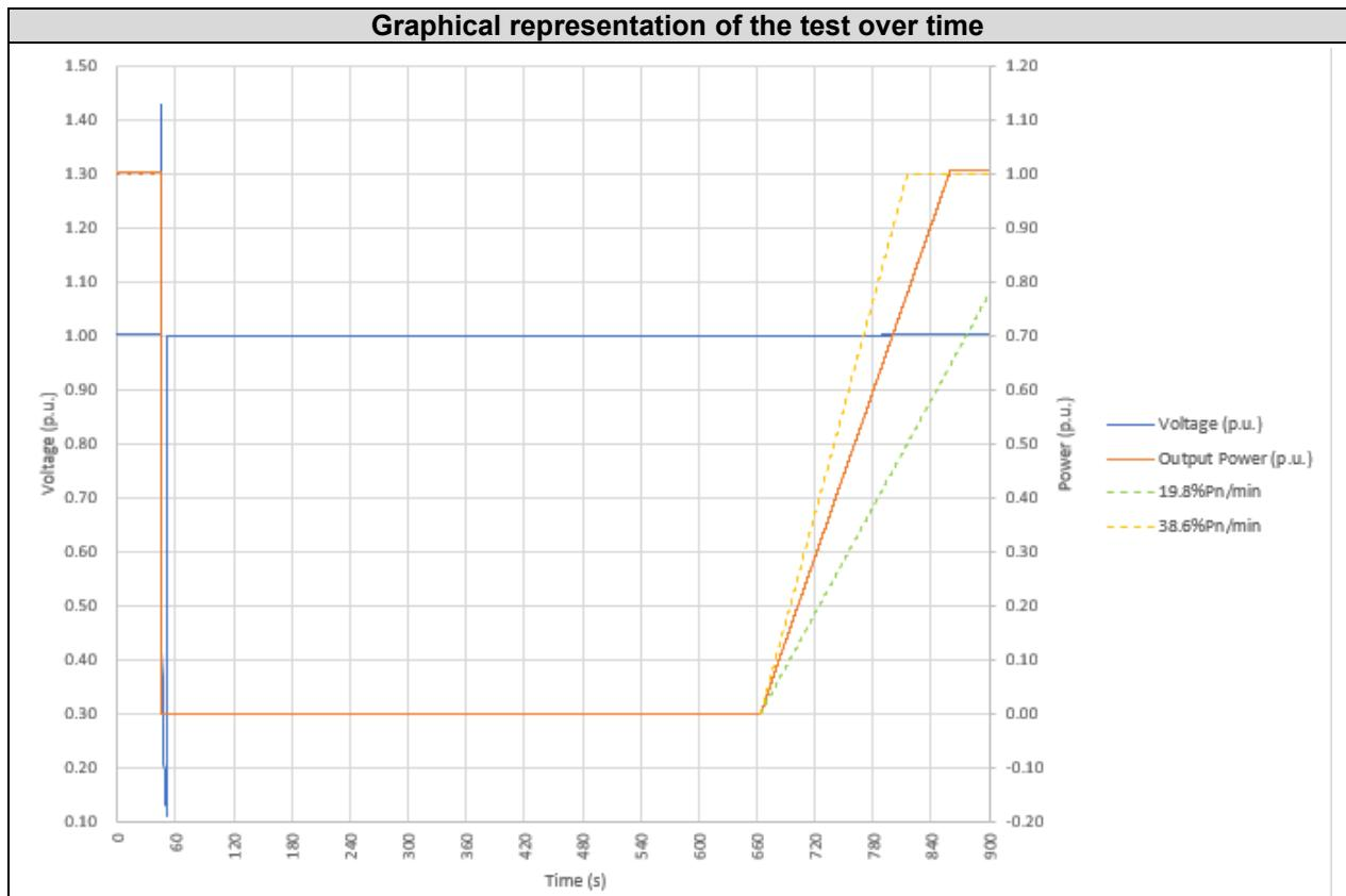
As it can be seen in the graph above, the active power gradient has been done according with option 1 of FGW Rev.25 as seen in the picture below:
