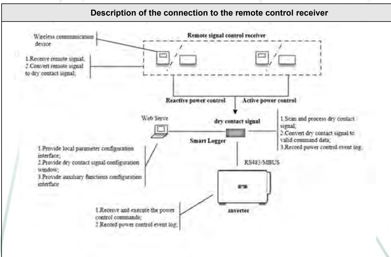
A generating station can receive the signal from the State Load Dispatch Centre or Regional Load Dispatch Centre for regulation of the active and reactive power output using the Smart Logger (data acquisition device).
