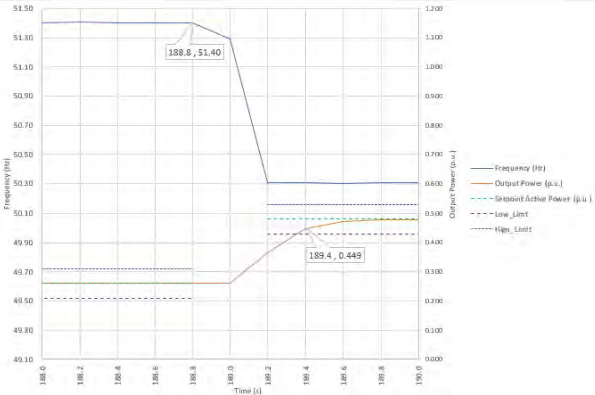
dP(f) desired: 40.0% P<sub>ref</sub>/HzdP(f) measured: 40.0% P<sub>ref</sub>/Hz
