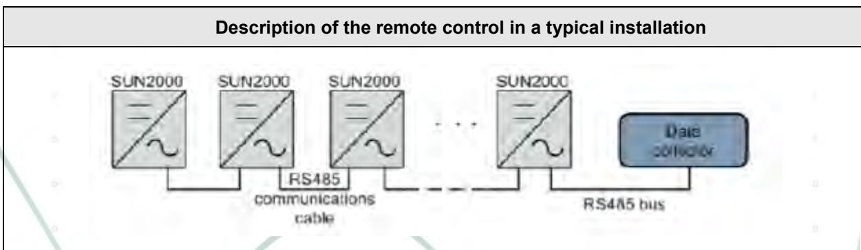
In the RS485 communication mode a SUN2000 system (including up to 30 units recommended by manufacturer each RS485 port) can be connected to the SmartLogger (data collector) via RS485 bus.
