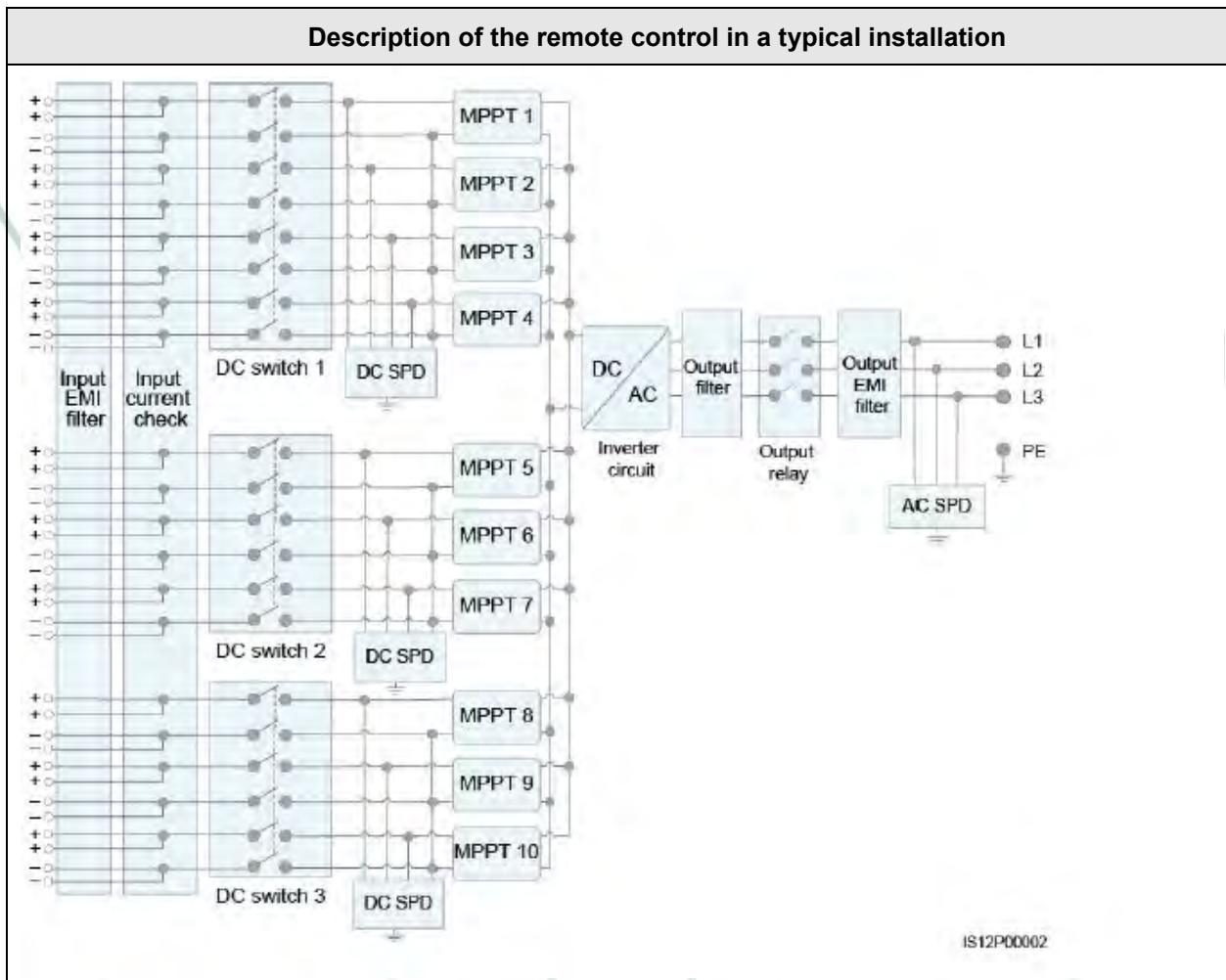
The SUN2000 receives inputs from eight PV strings. Then the inputs are grouped into four MPPT routes inside the SUN2000 to track the maximum power point of the PV strings. The DC power is then converted into three-phase AC power through an inverter circuit. Surge protection is supported on both the DC and AC sides.
