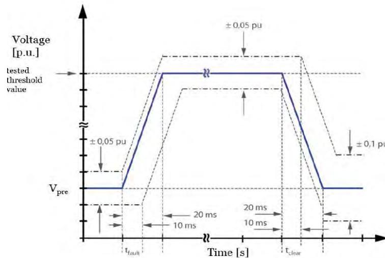
Fig. 4-27: Tolerances for overvoltage tests [2]
