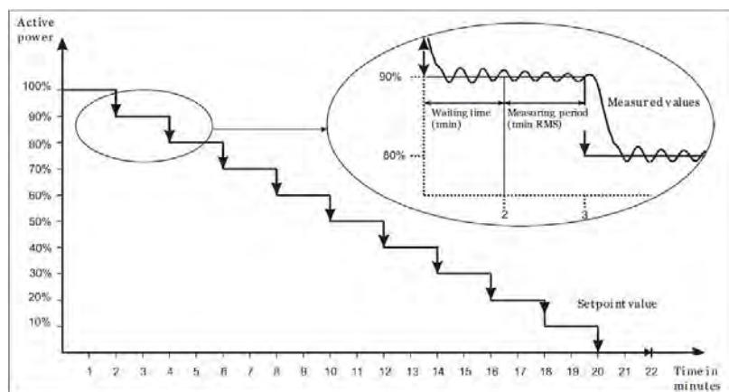
The active power and the reactive power have been represented in the positive phase sequence system and as 200 ms means for every setpoint step.
