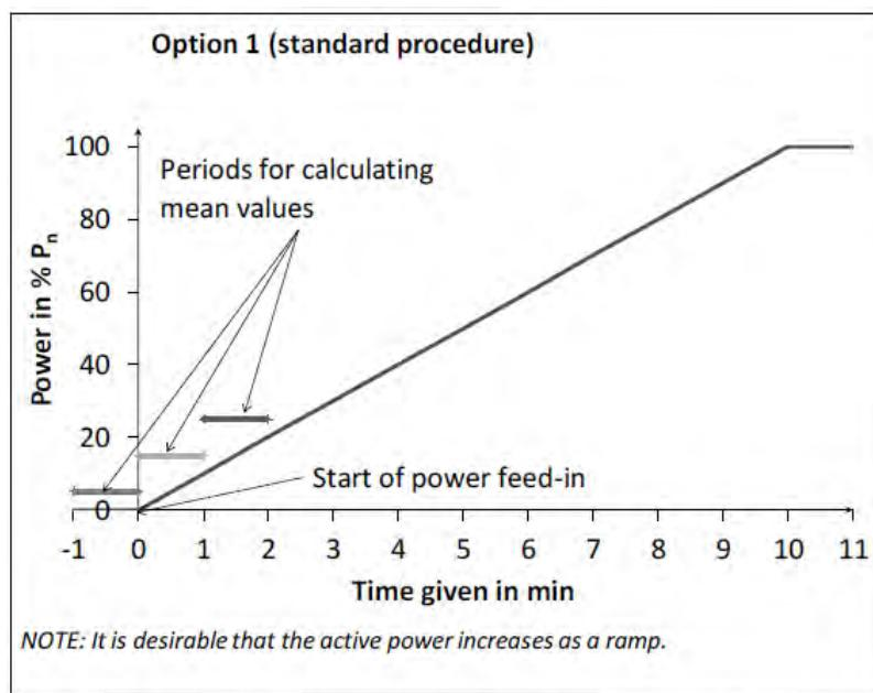
Fig. 4-9: Example with the first averaging interval 60 s before power increase
