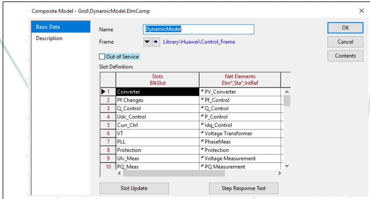
This controller block allows the user to configurate main adjustable parameters of the simulated conversion system for LVRT/HVRT tests.
