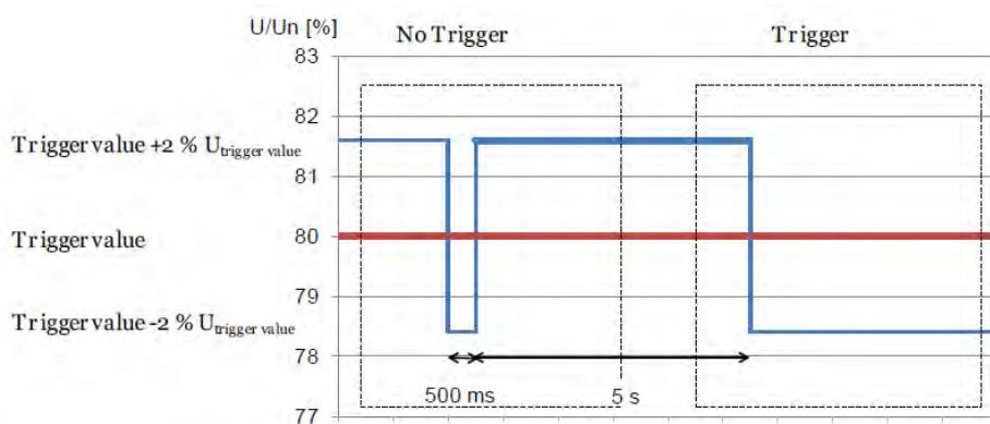
Fig. 4-24: Resetting ratio test for undervoltage protection
