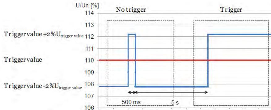
Fig. 4-23: Resetting ratio test for overvoltage protection
